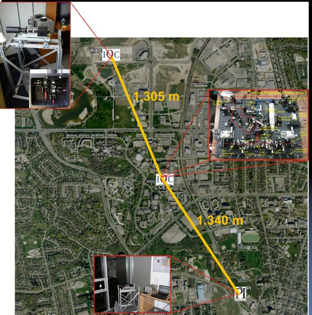
Sender telescopes and source remotely controlled by Alice or Bob (after initial alignment)
