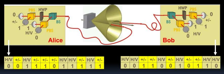
Polarization-Entangled Photons are created, coupled into optical fibres and sent to Alice and Bob
