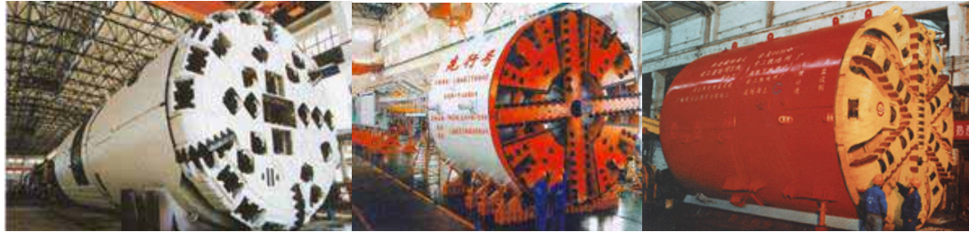
Rock tunneling machine
