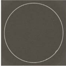
FIGURE 3.42 (a) Optical image of contact lens (note defects on the boundary at 4 and 5 o'clock). (b) Sobel gradient. (Original image courtesy of Peric Sites, Perceptics Corporation.)
